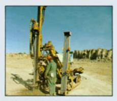
The CM-351 is a compact, powerful rig for drifter or downhole drilling of 64-140-mm (2½ to 5½") blastholes. Fixed-length boom. Its 2.2-m (7'3") width makes it easy to transport.
