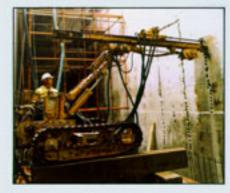
The LM-100 is ideal for small jobs in confined places; it makes fast work of holes 44-64 mm (1¾ to 2½"). Compact, but uses a 3-m (10-ft.) rod change.
