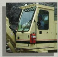
level at the operator's ear with the door and sliding window closed is 80 dBA.
