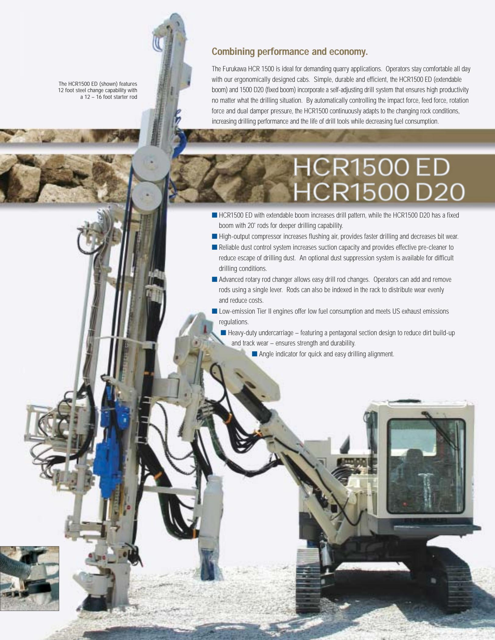
The HCR1500 ED (shown) features 12 foot steel change capability with a 12 – 16 foot starter rod
